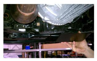
**STEP 5:** Install the (4) nuts onto the sub frame studs and tighten.
