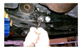
**STEP 3:** Remove the rear support brace from the sub frame studs.
